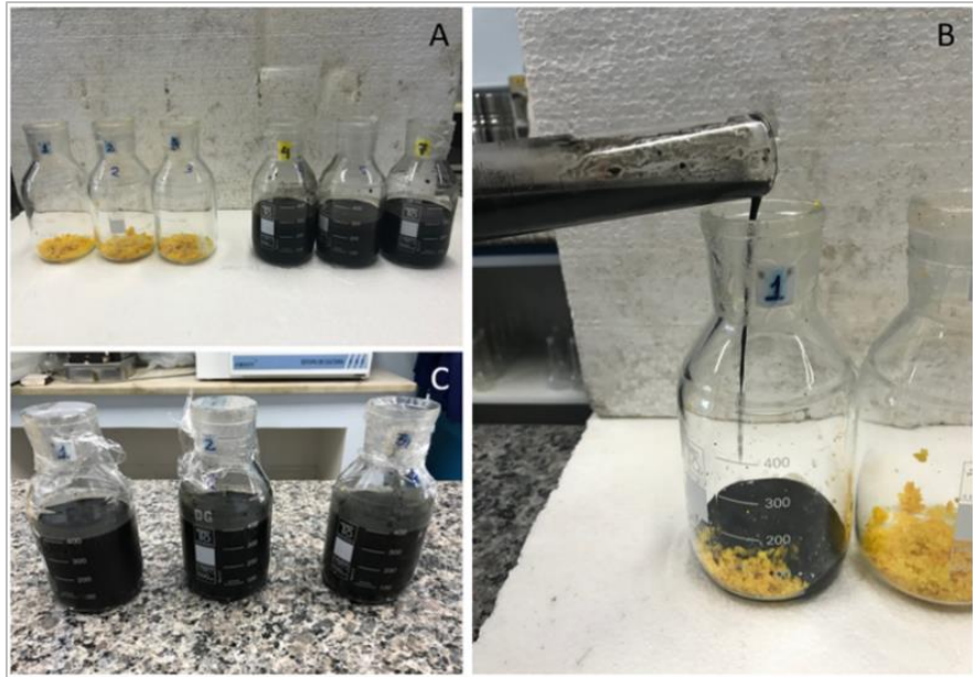
Figure 2: Preparation of the substrate-sludge mixture for the BMP test
