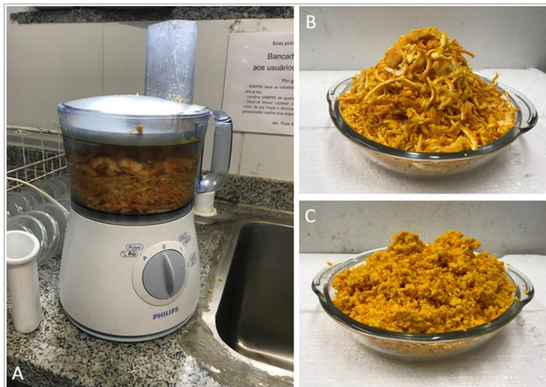
Figure 1: Crushing the substrate. A) Food multiprocessor; B) Sliced peel; C) Crushed peel
