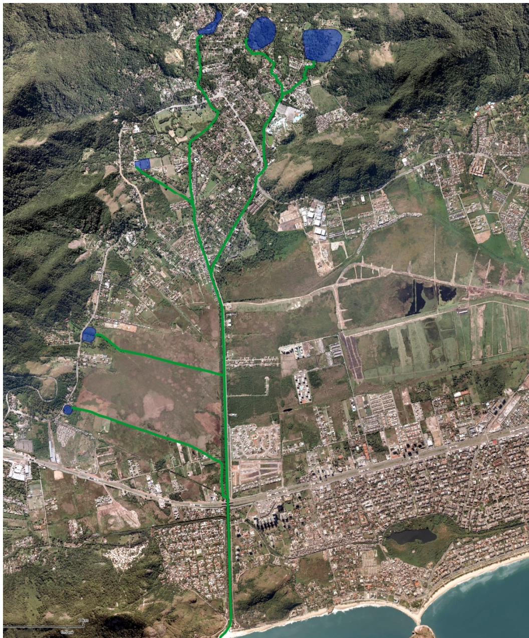
Figure 32: Area in study with the implementation of the 6 lagoons and its link with Sernambetiba Canal and flow into the sea. Source: GeoRio Portal – Digital Map
