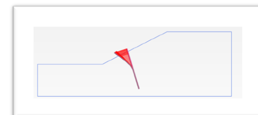
(h) Bamboo-pile 13 m length displacements
