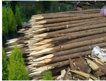
Figure 2.2 Rudimentary wood piles for soil stability
