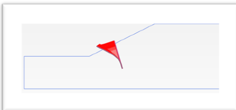
(g) Bamboo-pile 9 m length displacements
